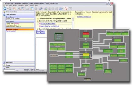
INTERLOCKS® modeling and simulation tool is a cost-effective and efficient means to conduct this analysis. Using existing discrete event simulation and fault isolation, the tool automatically identifies every failure that produces the same set of symptom indications. Using a model of the actual system design, INTERLOCKS is capable of finding interactions within the system that are not readily apparent using traditional methods. The engineer can use the tool to perform ambiguity analysis by:
